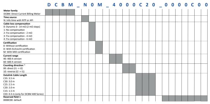
Note: 1) Current flow direction for imported energy registration. For example, DCBM\_N0M\_4000C20\_0000C00 registers imported energy when current flows from I1 terminal to I2 terminal. Below figure shows identification of the terminals.
